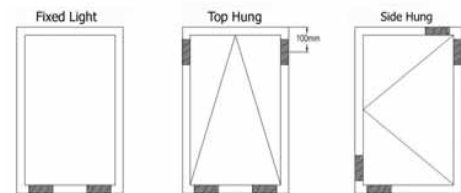
All spacer blocks are set 100mm in from the edge of the glazed units to the centre of the spacer block.
